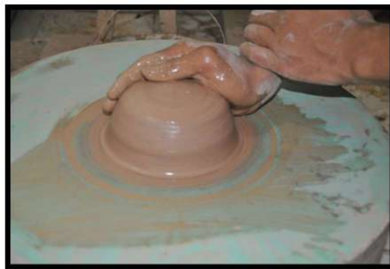
Gambar 18. Centering (Foto :Hendratno 2016)
